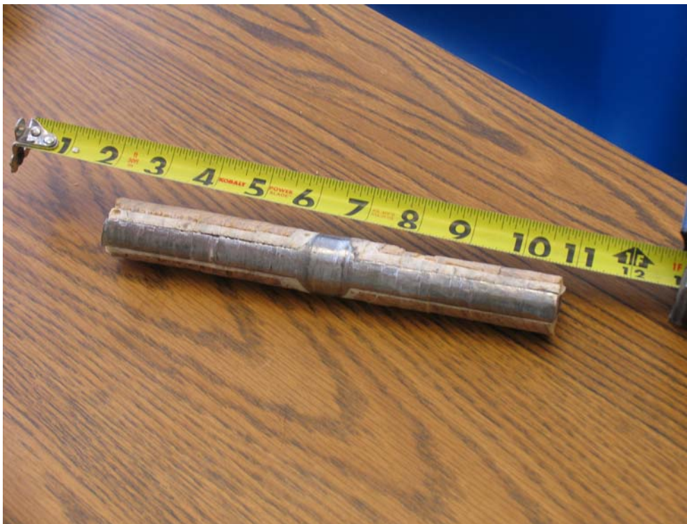
Figure 13. Core removed from arch at “Z” hanger. The center kerf plate is at the center of the member.
